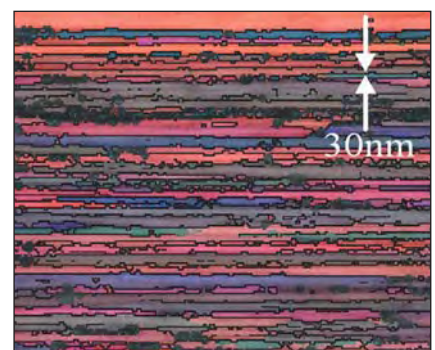
Fig. 4 — (top) Comparison of EBSD patterns collected from mechanically and Cross Section Polisher (center) prepared samples of steel cord; (bottom) EBSD map of the CP sample.
