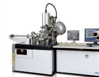
JAMP-9510F field emission Auger microprobe
